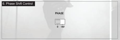
Allows you to change the phase of your subwoofer from 0 to 180 degrees to help compensate for timing differences between drivers.
